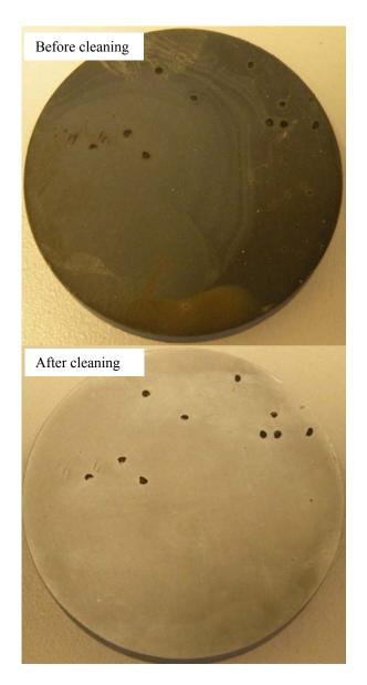
Figure 6.19 View of the experiment sample #1 after 25 days exposure with corrosion product layers and without corrosion product layers at test conditions 25°C, pH 5, 1 wt% NaCl solution saturated with CO<sub>2</sub>.
