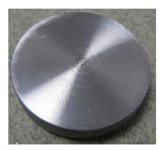
Figure 4.2 View of an API 5L X65 mild steel experiment specimen.
