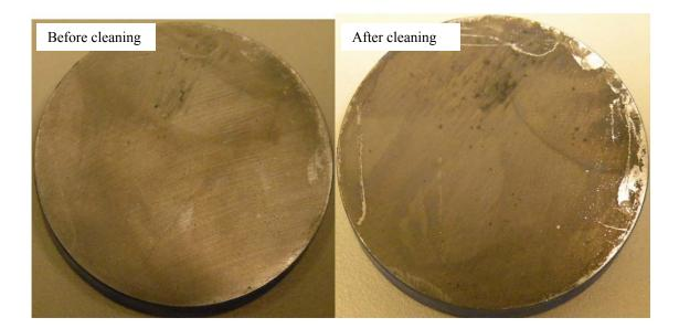
Figure 6.41 View of the experiment specimen after 14 days exposure at test conditions: 25°C, pH 5, 1 wt% NaCl solution saturated with CO<sub>2</sub>.
