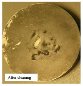
Figure 6.15 View of the steel surface after 9 days exposure at test conditions 25°C, pH 5, 1 wt% NaCl solution saturated with CO<sub>2</sub>.
