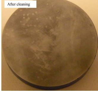
Figure 6.49 View of the experiment specimen #1 after 14 days exposure at test condition: 25°C, pH 5, 1 wt% NaCl solution saturated with CO<sub>2</sub>.
