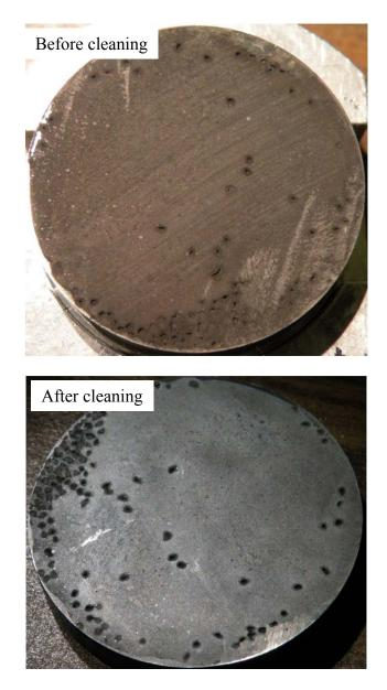
Figure 6.10 View of the steel surface showing a lot of pits after 40 days exposure at conditions 25°C, pH 5, 1 wt% NaCl solution saturated with CO<sub>2</sub>.
